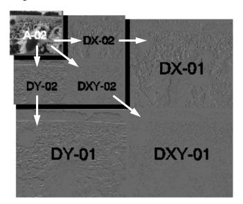
*Figure 3: Example of a 2-Level, 2-dimensional Wavelet Transformation*
