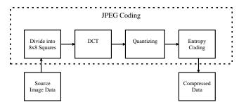
Figure 1 Simplified JPEG Coding Scheme for lossy compression
